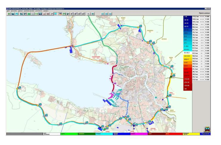
Depending on the hazard level ITS may decide only to inform road users about meteorological hazards, or to reduce the speed limit. The ITS provides information and management interaction with road users using variable information signs and placards.
