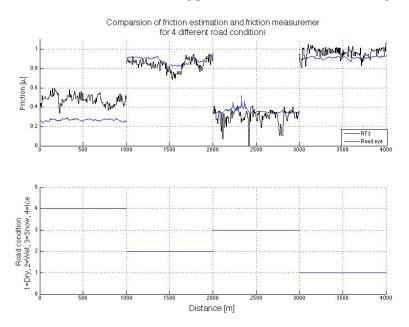
Figure 5. Comparison of friction estimation and friction measurement methods for different road conditions.
