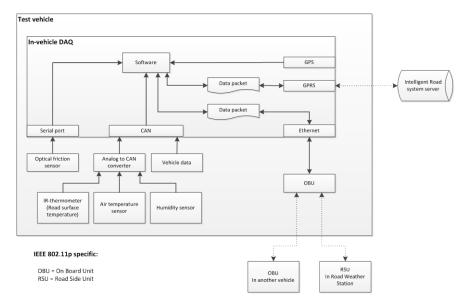
Figure 2. Description of a basic in-vehicle DAQ system setup.
