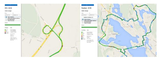
Figure 4. Friction view (RT3) on the left and surface condition view (Road Eye) on the right side.
