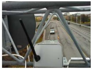
Figure 5. A laser radar affixed onto a gantry in the pilot site for measuring traffic and road data.
