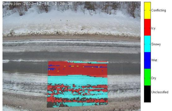
Figure 6. Background image taken with ordinary visual camera system. A classification image made from NIR camera data is overlayed on a part of the visual image. It can be seen that different road conditions are detected on the road surface.
