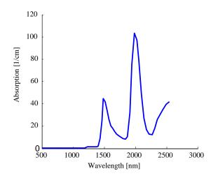
Figure 2. Water absorbtion in the region 500 to 2500 nm [5]. It can be seen that there are some peaks in the absorption that may be used to detect water.
