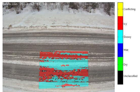
Figure 7. A classification image made from NIR camera data is overlayed on a part of a visual image. It can be seen that different road conditions are detected on the road surface.
