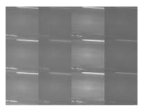
Figure 4. Image retrieved from NIR camera unit. Each row represents images with a specific exposure time. Each coloumn represents a wavelength band.
