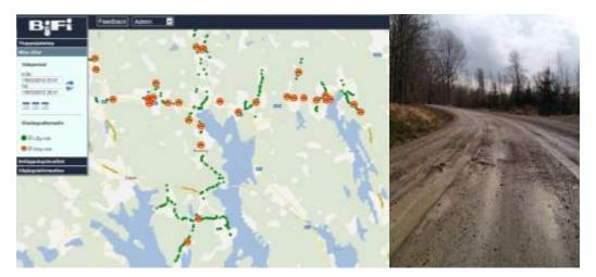
Figure 2.Display of frost thaw situation and example of how a typical gravel road can look like during these conditions..
