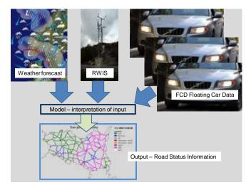
Figure 1. RSI – for winter road conditions, where input from different sources makes it possible to improve the information to maintenamce operators.
