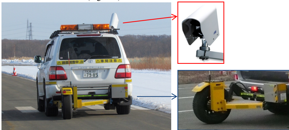
Figure 1. Test vehicle equipped with the CFT and the DSC111.
