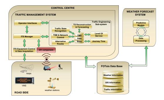
Figure 1. FOTsis highway control center structure.
